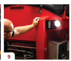
**STROBE & WORK LIGHTS**Check that strobe and work lights are functioning properly.
