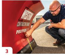
**CUTTING EDGES**Check for wear and align for best performance and structural integrity.
