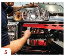
**HEADLIGHTS**Adjust plow headlights for proper aim.
