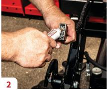
**CONNECTIONS**Clean and tighten all electrical connections. Apply dielectric grease.
