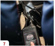
**HYDRAULICS**Drain system and refill with fluid annually. In-season, check levels.
