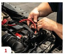
**BATTERY**Inspect and test the battery and charging system.
