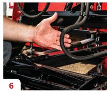
**HOSES**Check hoses for leaks, cracks and damage. Replace as needed.
