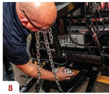
**PAINT**Check exposed areas and repaint to prevent corrosion.
