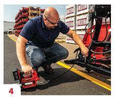
**FITTINGS**Check to make sure they are tight and don't leak. Lubricate as recommended.
