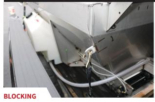
The spreader must have blocking between the front of the sill and the bed of the truck to maintain support and proper spreader position in the vehicle.
