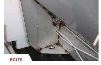
The spreader must be bolted to the vehicle frame. Do not rely on tie-down chains or straps alone to hold the spreader in the vehicle.
