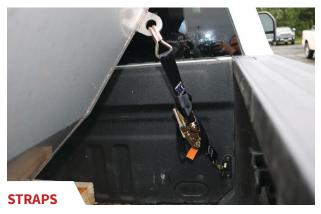
Periodically check all spreader to frame fasteners and hold down straps for tightness and adjust as necessary.
