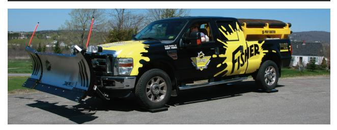
The final check is to ensure that the front axle weight distribution is not exceeded with all of the equipment, driver and payload in place.
