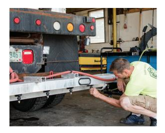
**Fix it fast:** Keep an equipment "first aid" kit handy. At minimum, every truck should have basic hand tools and a hydraulic hose repair kit.
